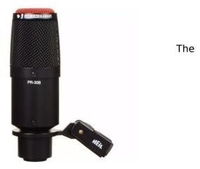
microphone's supercardioid pickup pattern rejects off-axis noise, focusing on the sounds in front of it. The steel body and internal hum bucking coil shield the microphone, making it safe for use near video monitors and noisy lighting fixtures. An internal Sorbothane shock mount decouples the microphone's dynamic element from the body to reduce the effects of handling noise.
