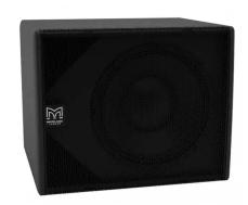
response of 48Hz-150Hz  $\pm$  3dB, the ultra-compact size of the CSX112 makes it an ideal partner for CDD Series systems where space is at a premium or where the subwoofers need to be hidden. The enclosure is constructed from high-density MDF and has an impact-resistant finish, while the driver is protected by a rigid perforated steel grille, which is pre-curved to withstand physical damage.
