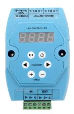
Controller allows for DMX or stand-alone control of HL1606 based LED Ribbons. Allows for full control of LED Ribbons over DMX or in stand-alone mode control can be achieved of any of the built-in sequences such as jumpy changing, comet trail, gradual changing, fading, color wash or others.
